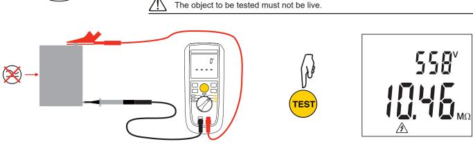
Press the **TEST** button and keep it pressed until the measurement is stable. The A symbol indicates that the instrument is generating a hazardous voltage.
