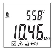
The alarm thresholds can be programmed (see §3.9). There is one for each test voltage.
