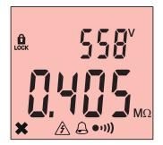
On the other hand, if the measurement is below the threshold, the instrument emits a continuous beep, the backlighting lights red, and the **X** symbol is displayed.
