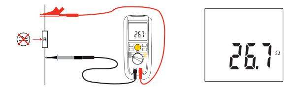
To make sure that there is no voltage, you can make a voltage measurement before the continuity measurement. Otherwise, the instrument will report the presence of a voltage if there is one.
