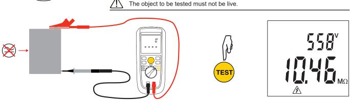
Press the **TEST** button and keep it pressed until the measurement is stable. The A symbol indicates that the instrument is generating a hazardous voltage.
