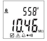
The alarm thresholds can be programmed (see §3.9). There is one for each test voltage.
