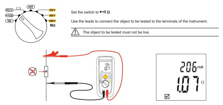
To make sure that there is no voltage, make a voltage measurement before the continuity measurement.
