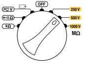
Set the switch to one of the  $M\Omega$  positions.
