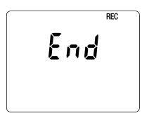
If during start-up the instrument displays the screen shown opposite, it means that a recording session has been brutally interrupted by a power outage.
