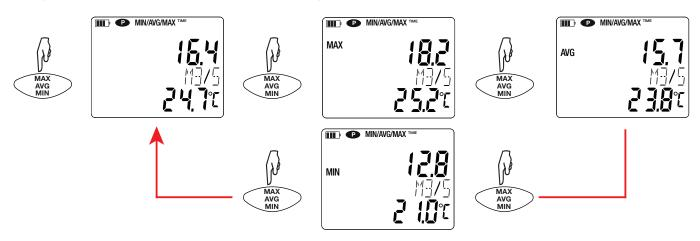
To exit from the MAX AVG MIN mode, long-press the MAX AVG MIN key.
