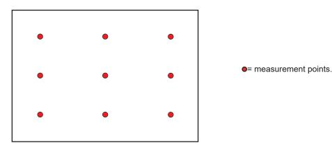
Place the sensor on the first measurement point and press the MEM key to record the value in memory. The counter is incremented.
