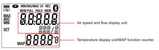
When the measurement exceeds the limits, the instrument displays OL.
