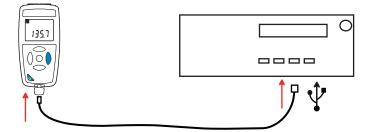
It is treated as a USB key and you can access its content. But to read the records, you must use the Data Logger Transfer software.
