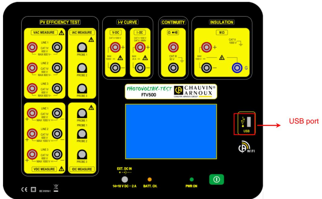
The instrument can read and write from any key with FAT32 or NTFS file system.
