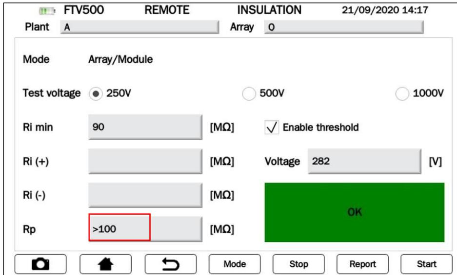
Figure 14.7.5-12 Measurement in ARRAY/MODULE mode
