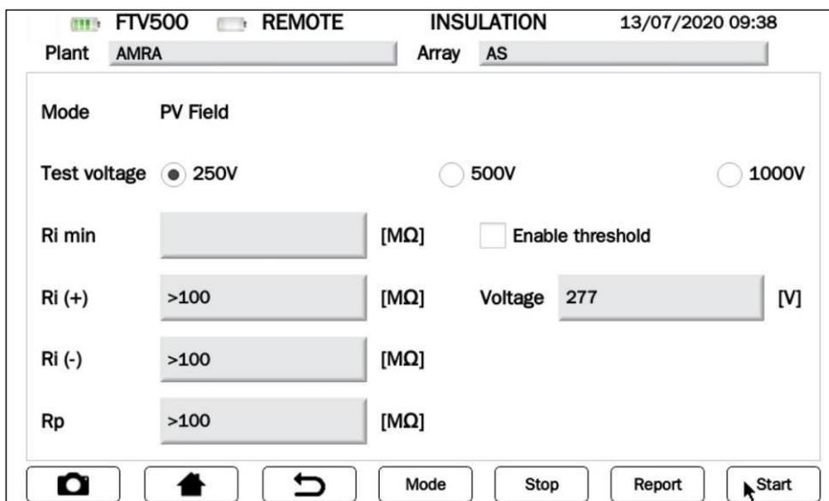
Figure 14.7.5-8 Insulation measurement in PV FIELD mode
