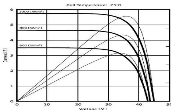
On each characteristic curve there is one and only one point whereby the transfer of power to a hypothetical load powered by the photovoltaic module is maximized. The maximum power point corresponds to the voltage-current pair such that the product  $V * I$  is maximum, where  $V$  is the value of the voltage at the module' poles and  $I$  is the current that circulates in the circuit obtained by closing the module on a hypothetical load .
