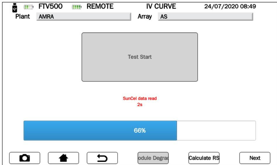
Figure 14.7.3-11 Data acquisition for drawing I-V curve
