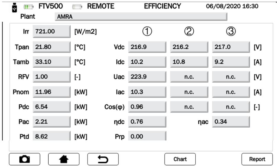
Figure 14.7.1-9 Efficiency measurement display
