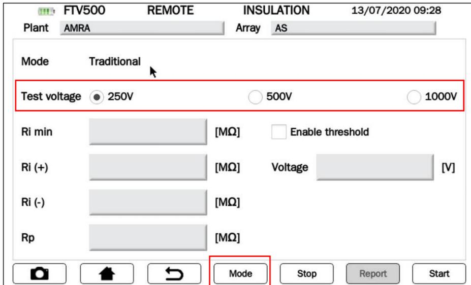
Figure 14.7.5-1 Insulation measurement
