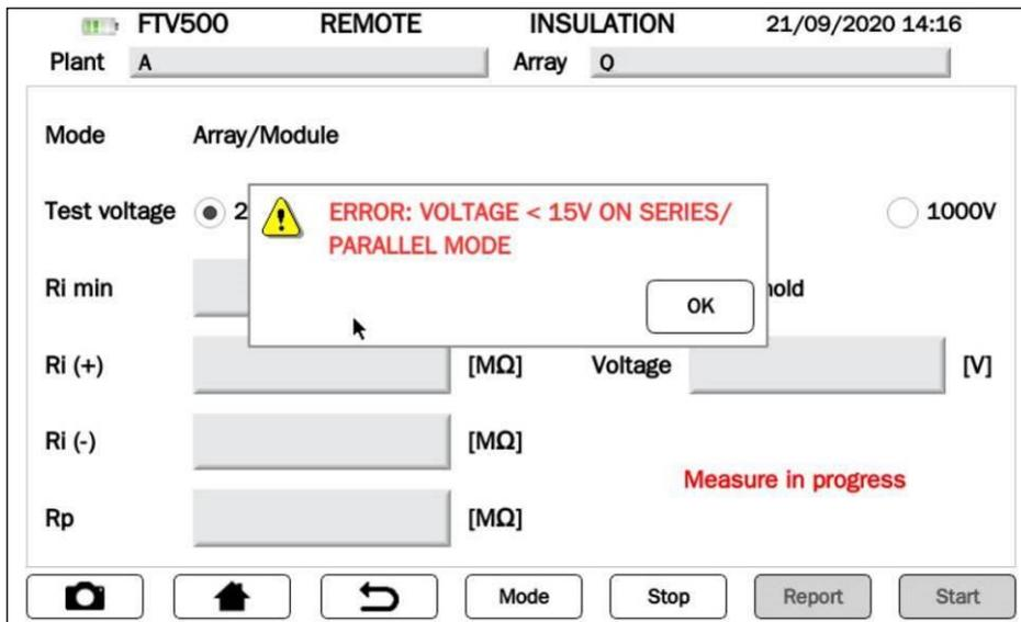
Figure 14.7.5-13: Error when voltage is less than 15V
