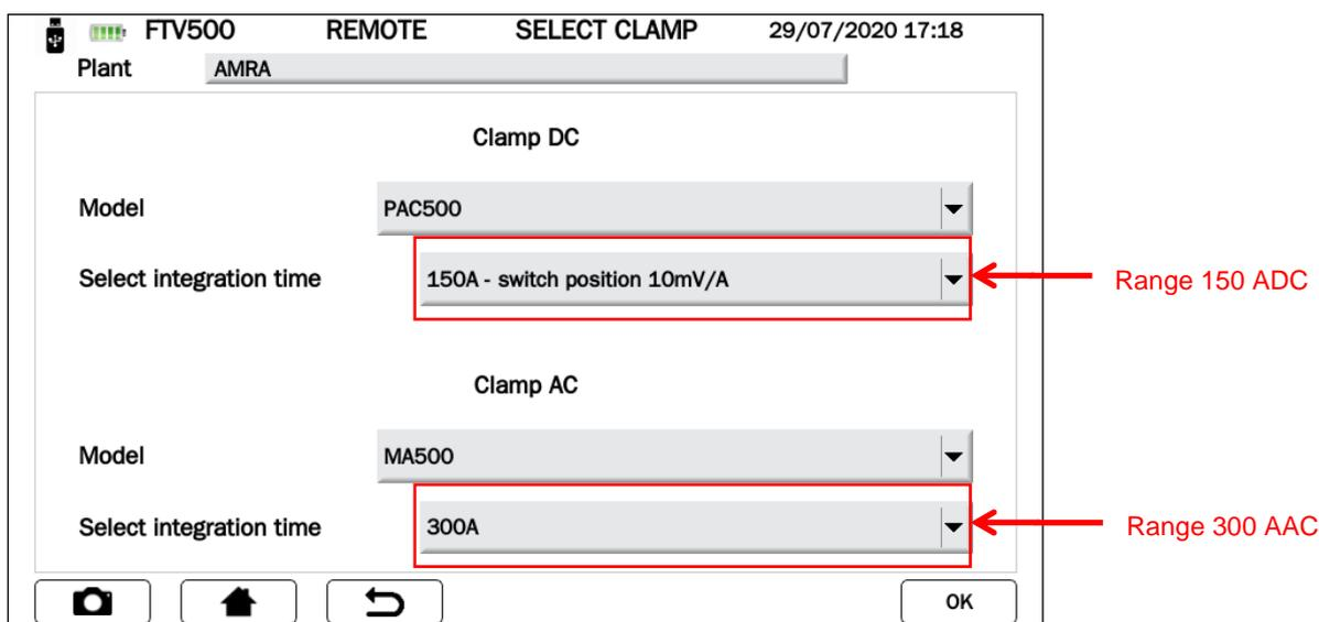
Figure 14.7.2-4 Clamp meter range selection (lower ranges)
