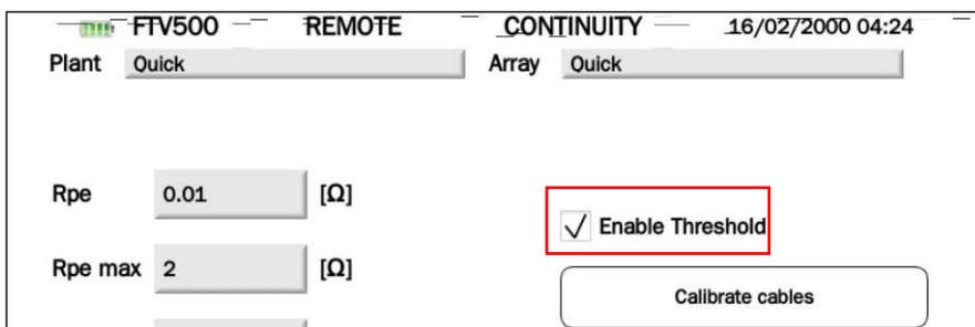
Figure 14.7.5.2-6 Screen; Resistance treshold in continuity test enabled
