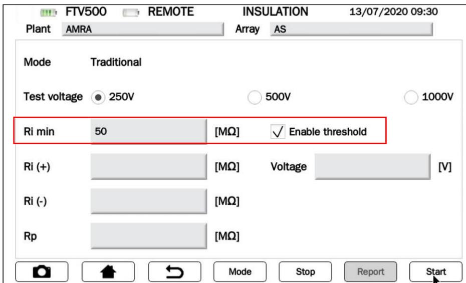
Figure 14.7.5-4 Entering and enabling an insulation resistance treshold
