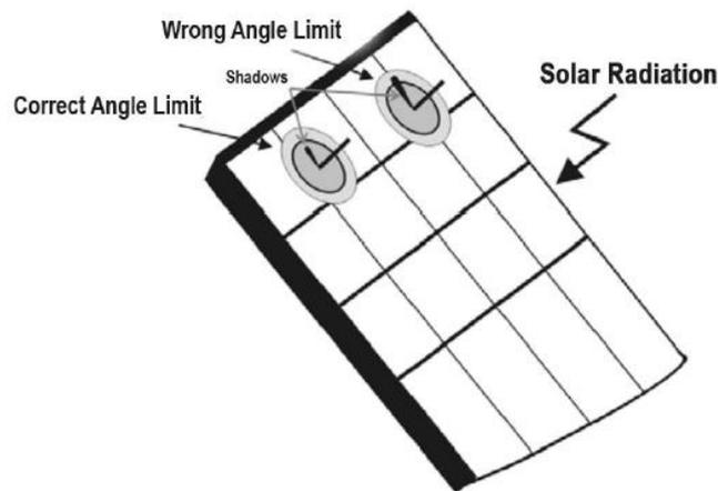
**REMOTE UNIT:** the Remote Unit must be positioned correctly on the same plane as the modules to be tested, it is also necessary to ensure that there are no shading, in order to avoid fake measurements.
