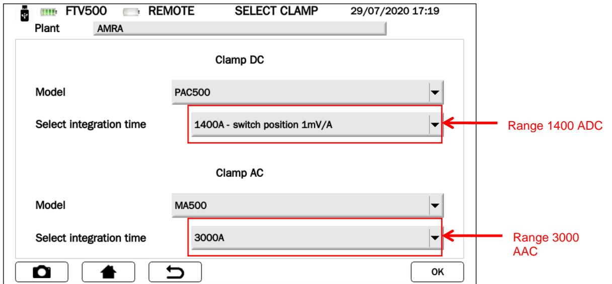
Figure 14.7.2-5 Clamp meter range selection (upper ranges)
