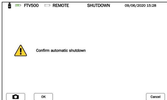
During the shutdown the display switches off immediately and the LED will switch off after approximately 20 s.
