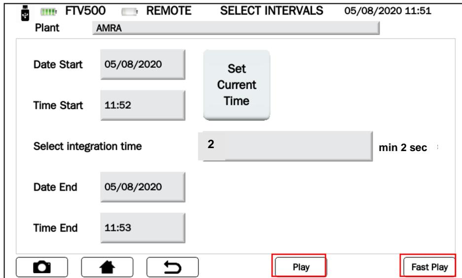
Figure 14.7.2-10 Datalogging programming menu
