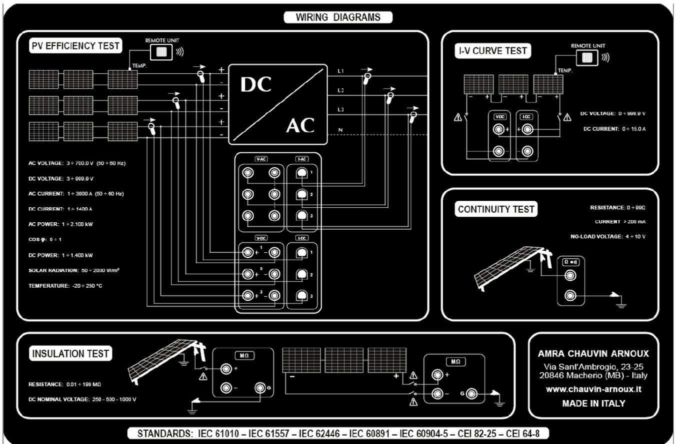
NOTE : If there is a neutral conductor, this has to be connected to the black V-AC input terminals. If there is no neutral conductor, these terminals have to be connected between each other.
