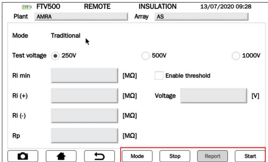
Figure 14.7.5-6 Insulation measurement start
